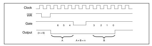
Figure 2-32. Mode 0 Timing Diagram
